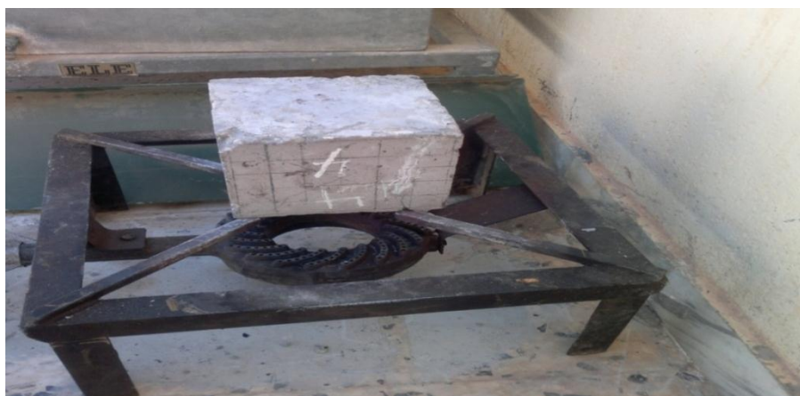
Fig. 2 Sample exposed to direct flame
