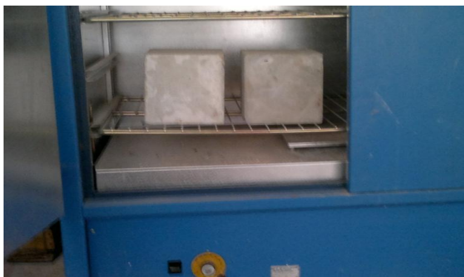
Fig. 6 Concrete specimens in the electrical oven
